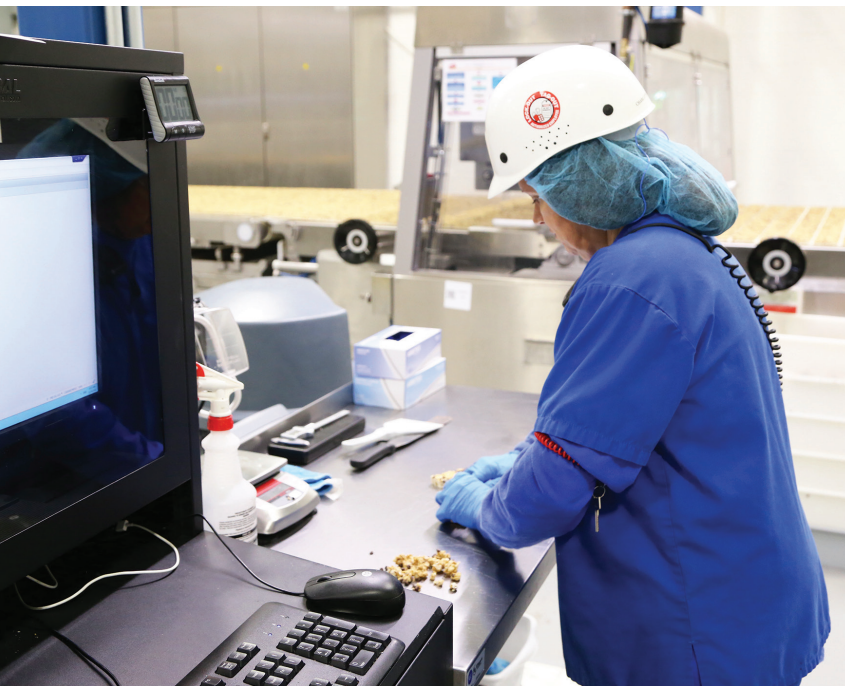
An operator takes samples after the guillotine to check for weight and make any necessary adjustments in the HMI.
