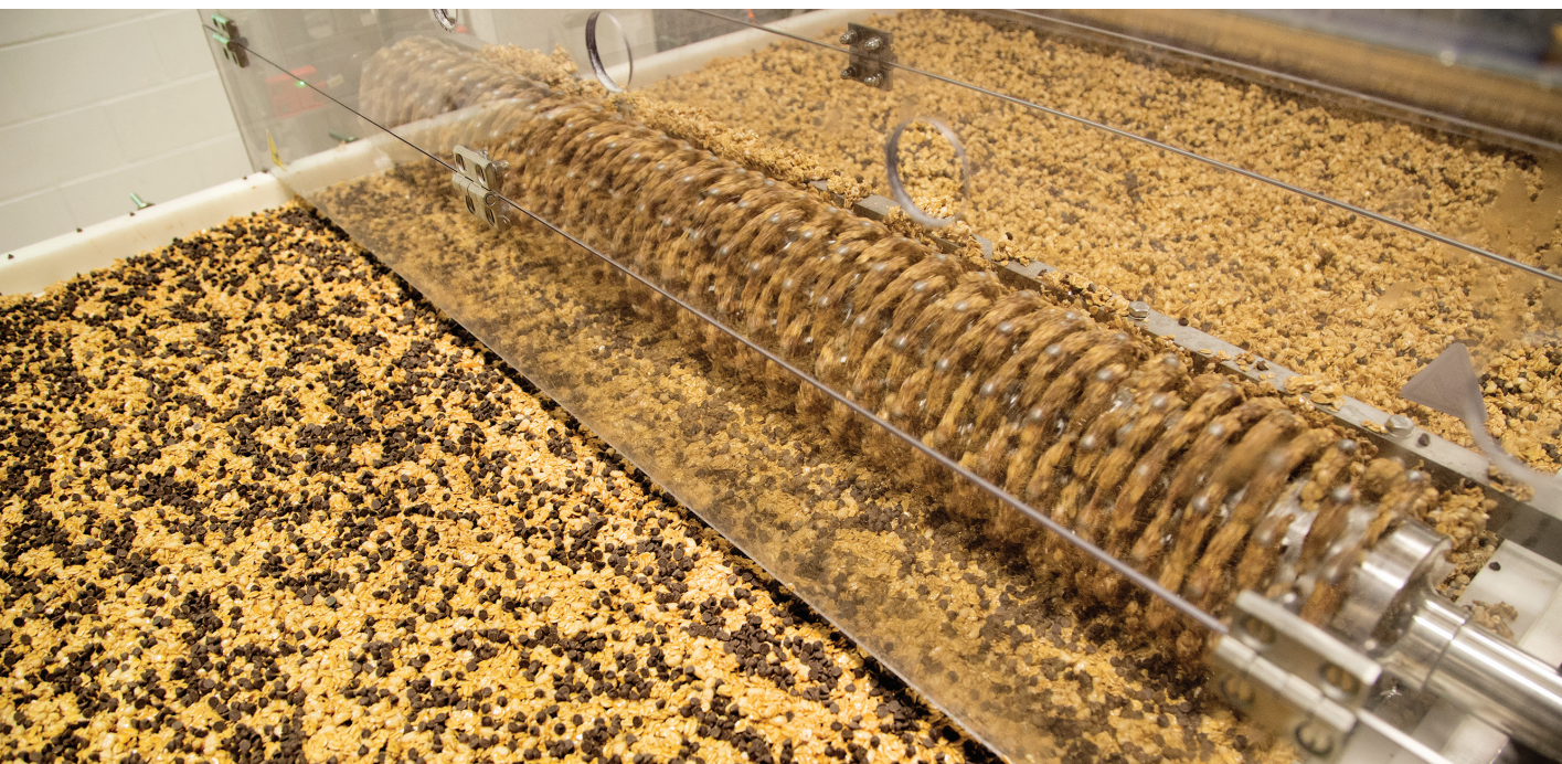
An inclusion wheel mixes in chocolate chips and ensures even distribution.
