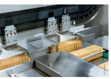
The slugs get tilted by 90 degrees before being handled by the XTS movers.
