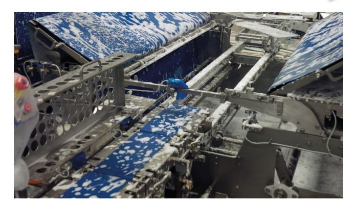
tion supports CIP (Cleaning In Place) operations and high-pressure washing with pressurized water and caustic foams.
