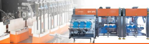
The Cavanna secondary packaging range is very wide and allows to form, fill and close cartons at high speed and high efficiency through carteasian robots, pick and place and innovative vision systems.
