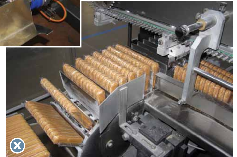
Versatile tooling. Photo above shows the tool used by the racetrack bucket-infeed system when primary packs are sent into secondary packaging on edge. Photo on the left shows tooling used when two or three primary packs are multipacked one on top of the other.
