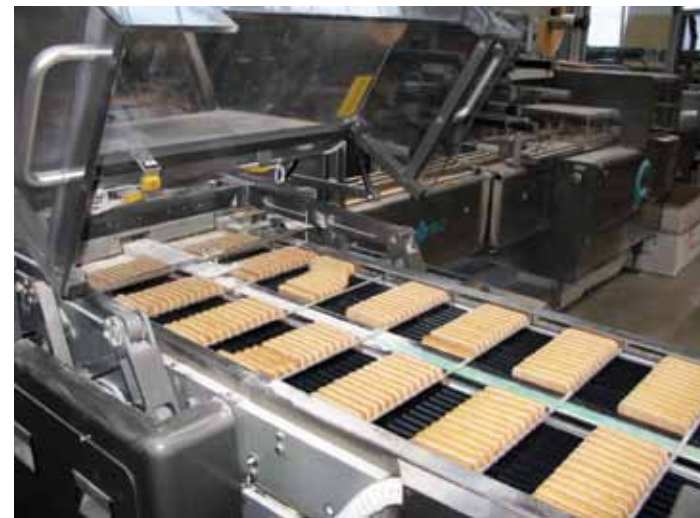
90-Degree transfer. Ladyfingers are conveyed to the servo driven 90-degree transfer device in parallel groups of 12. With each stroke, the transfer device gently pulls 24 ladyfingers onto a conveyor belt leading off at a right angle to primary flow wrapping.
